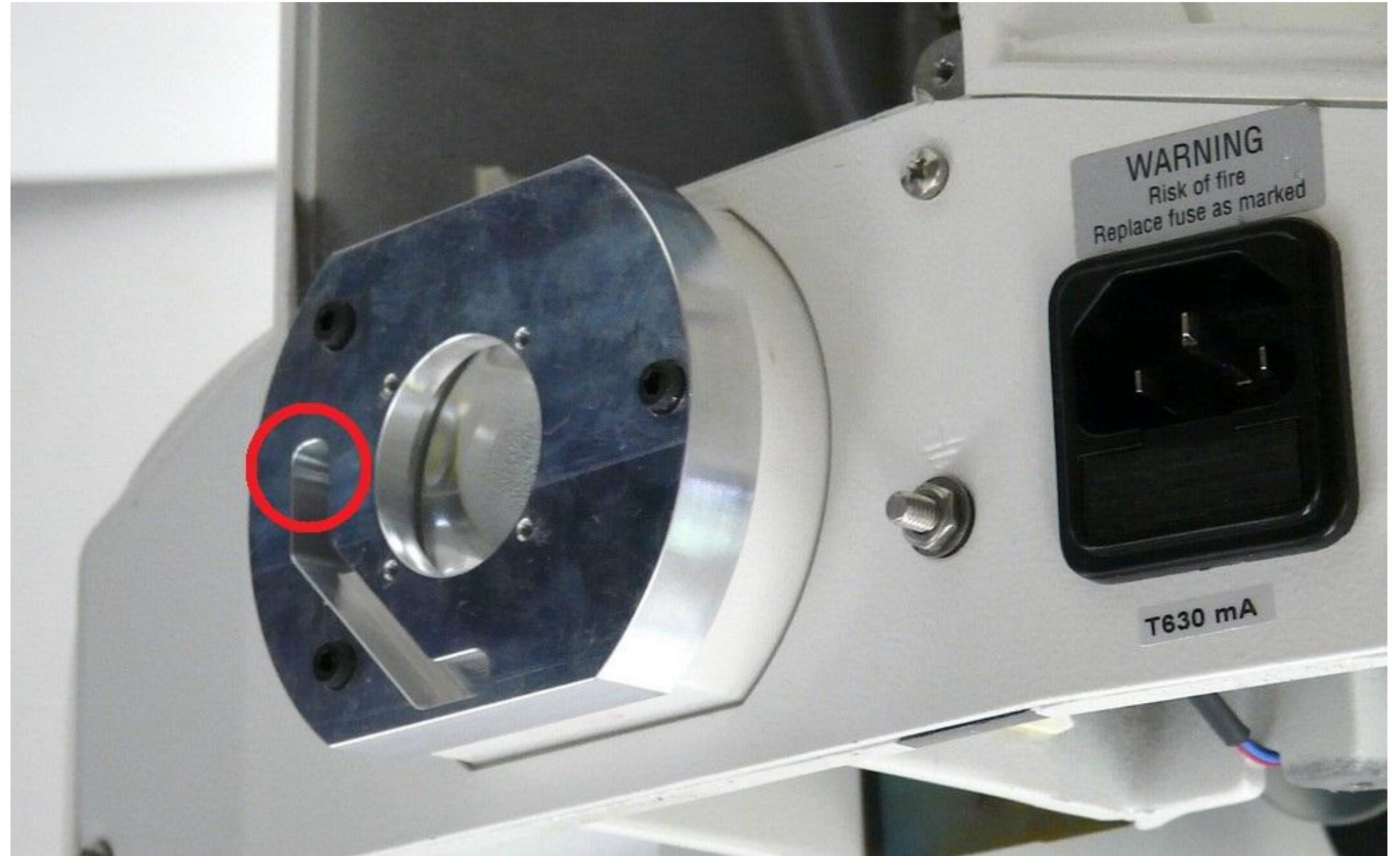
(3) Attach the adapter as shown. Use the M3 screws and the 2.5mm hex key. In the photo, the screws have just been started. See warning at right.
