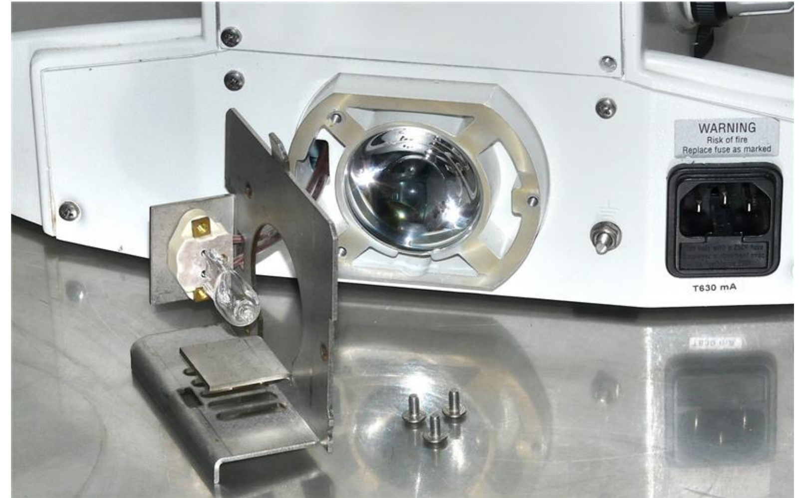
(2) Remove the three screws holding the lamp holder. Be aware that the lens can now fall out.
