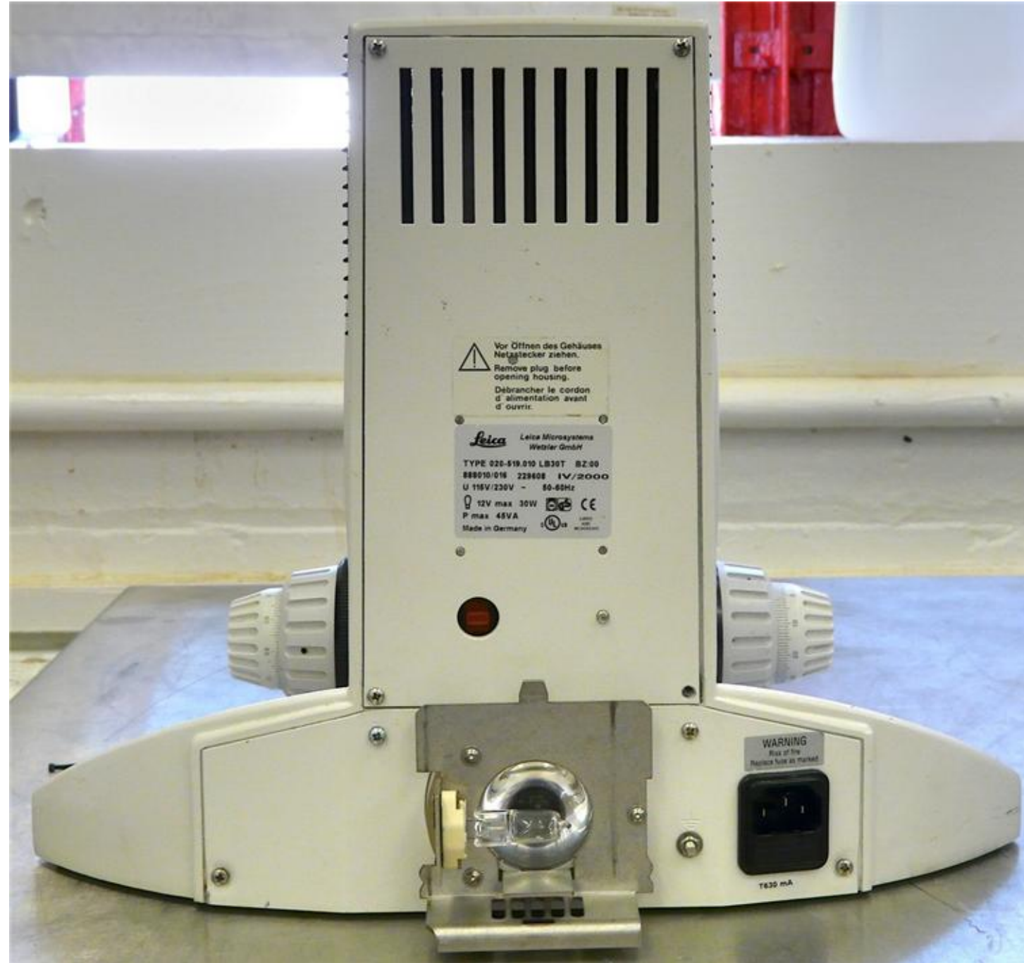
(1) Back of microscope with original illuminator housing removed, exposing the lamp holder.
