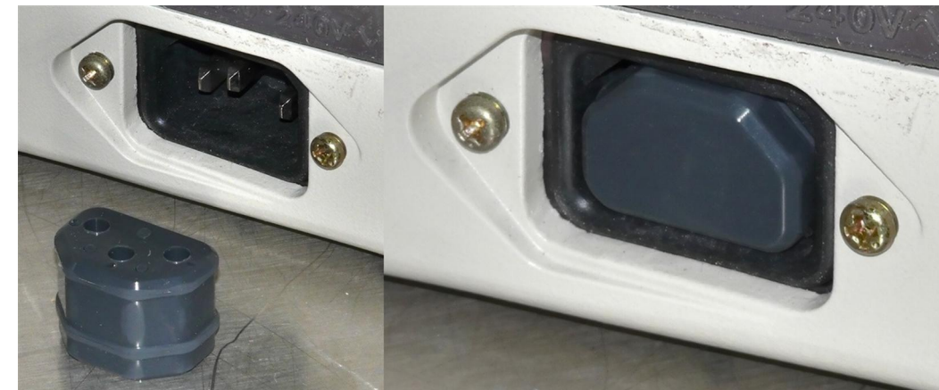
(2) Install PN 10736 rubber blocking plug in the AC receptacle as shown in the photos above (from a different microscope).
